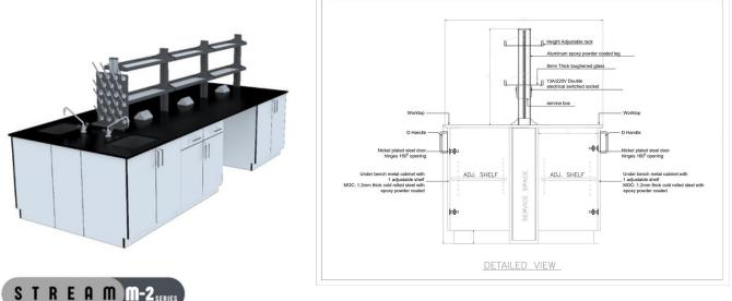
The STREAM- M2 series is designed with hygiene in mind, Worktops are supported on Metal H' Frame (made of 30 / 40 mm square tubes) which provides easy cleaning for floors. An ideal solution for hospitals or infection-control labs.
